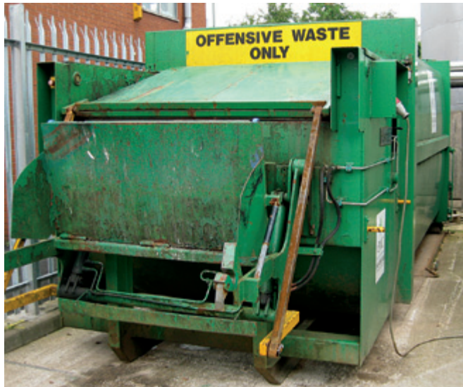
Mobile compaction unit
